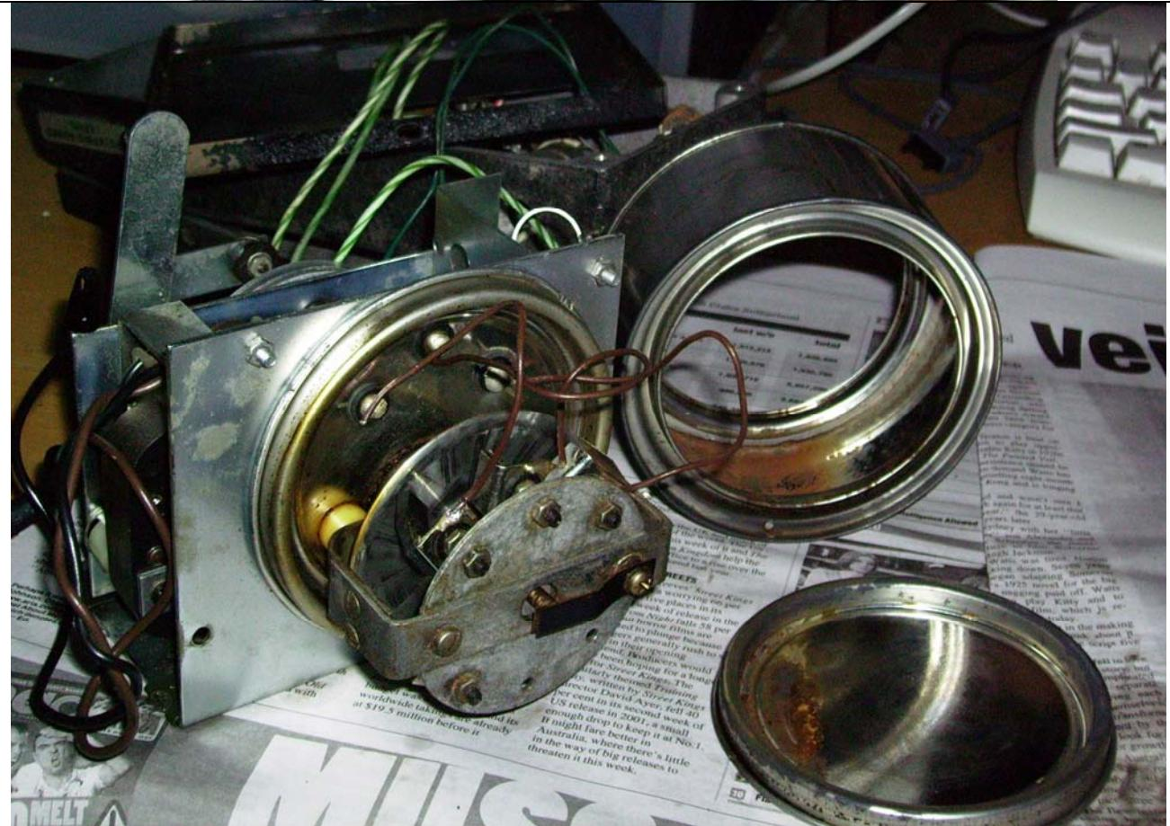
Operation with 110VAC 50Hz showed that motor worked, and power supply rails showed 67VDC and 13VDC, with the secondary (two red wires) at 46.7VAC unloaded. The transformer white wire is from a screen, and is soldered to the ground.
